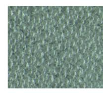
Foam structure in the microscope
