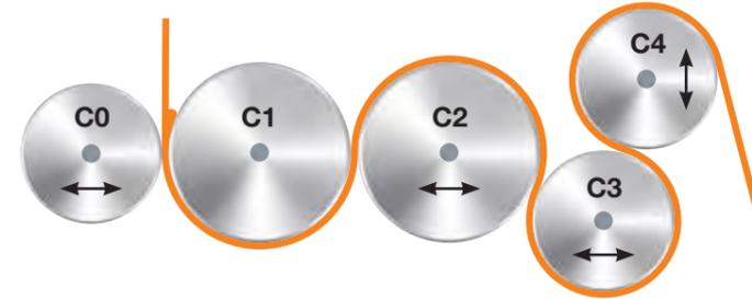
The roll stack technology from SML is characterised by precise temperature control **for effective sheet cooling** and the best operability.
