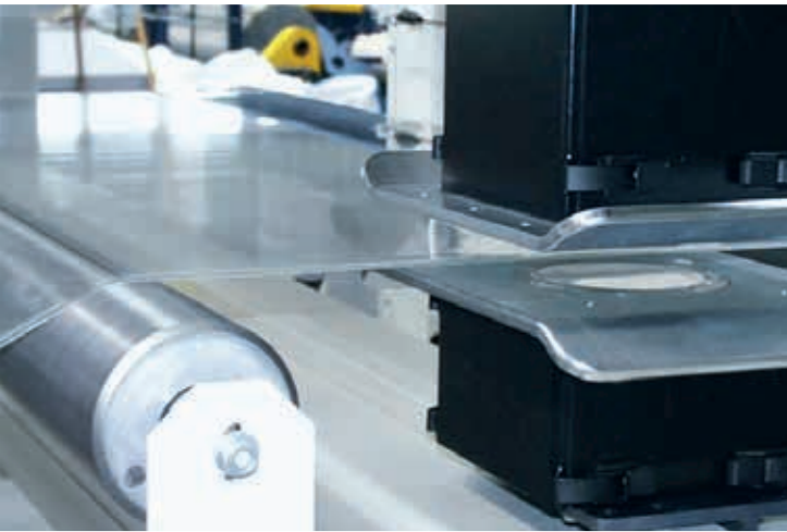
Inline thickness measuring unit with a Beta-ray sensor
