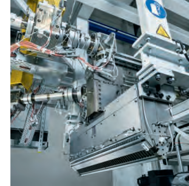
Tool unit with a melt pump, static mixer, feedblock and flat die
