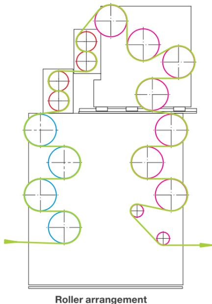
In the new MDO, rollers are arranged in the form of an inverted "U". This new layout is particularly advantageous with regard to straightforward roller insertion and removal to the outside of the inverted "U". All of the preheating, stretching, stabilising and cooling rollers can be exchanged very rapidly through rolling out onto an attachable installation device via lockable slits on the stretching unit's perimeter.
