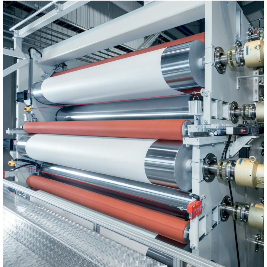
New MDO unit with an adjustable stretching gap
