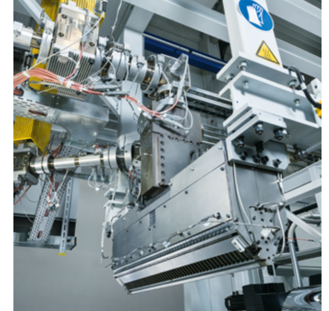
Tool unit with a melt pump, static mixer, feedblock and flat die
